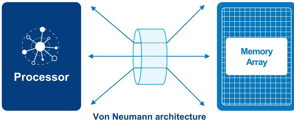
**Memory bottleneck** (or Memory wall) due to serial communication method between processor and memory area
